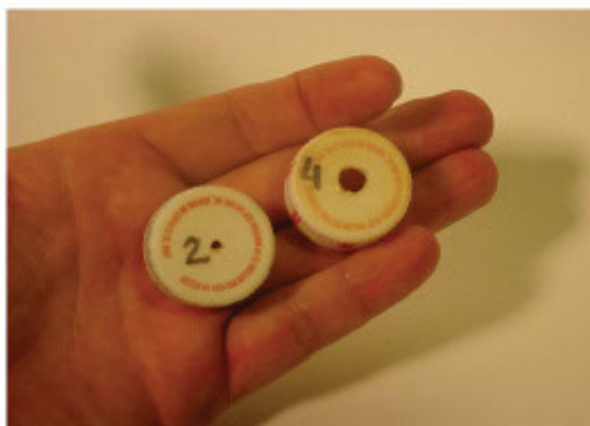
Cap with a \frac{1}{8} " hole and cap with a \frac{1}{4} " hole from our very first fountains 1
