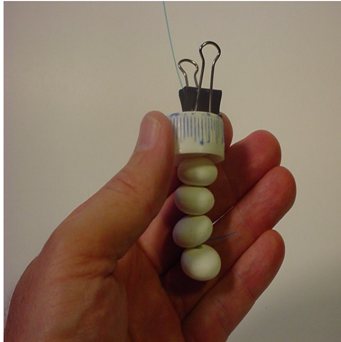
The cartridge: five Mentos hanging on fish line below the bottle cap
